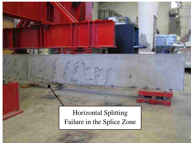
Figure 5.10 – Failed splice specimen
