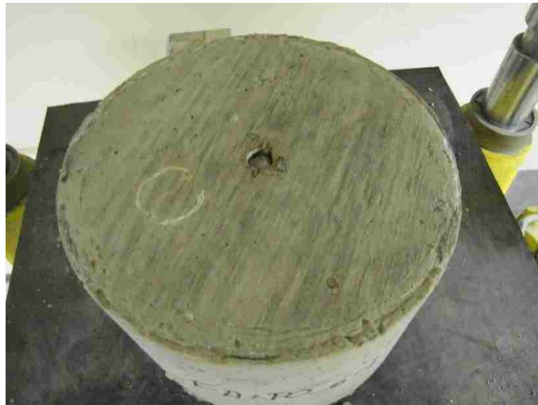
Figure 4.7 – Failed pull-out specimen
